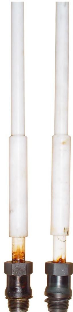
What you see here occurred within only a few hundred hours. The spark plugs have been so contaminated, have arced[flashed-over]-over so frequently that they are totally unsuitable for continuing use. They must be replaced.
