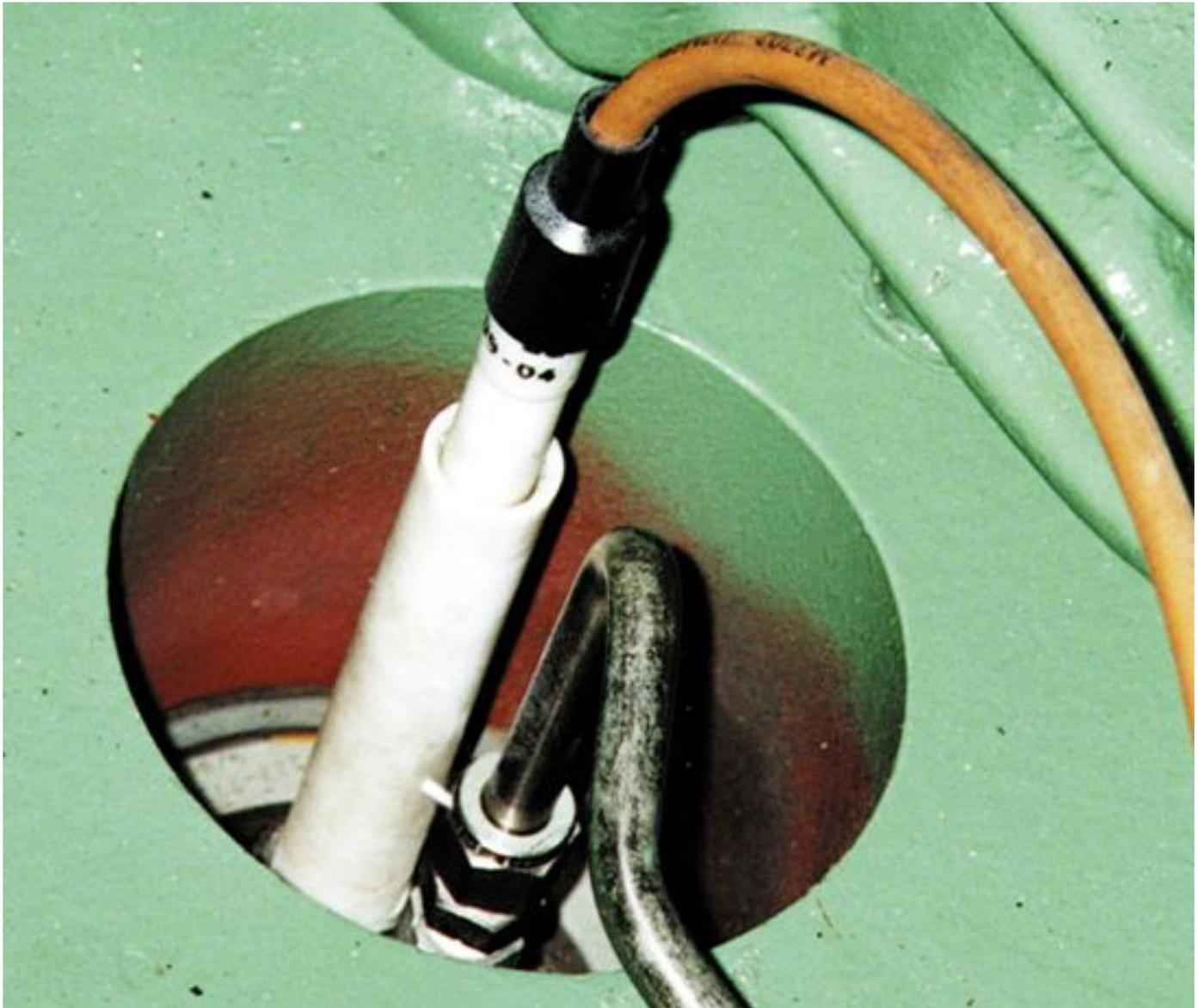
One way of thinking has it that short, conventional spark plugs used with a plastic[PTFE, for example] extension+boot assembly is the most cost-effective way to configure the high-voltage side of the electrical ignition system.
