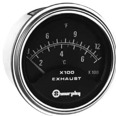
These Murphy analog pyrometers do not require power. NEVER apply vehicle voltage to pyrometer terminals, damage beyond repair will occur. Only the illuminating lamp requires voltage.
